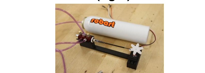
Fig 5: Complete pneumatic compression system: valve, tank, servo, tubes, and 3d-printed holder
